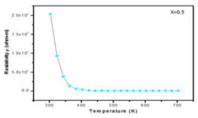
**Figure 9** (e) Temperature dependent resistivity curves for Mg<sub>(0.5)</sub>Cu<sub>(x)</sub>Zn<sub>(0.5-x)</sub>Fe<sub>2</sub>O<sub>4</sub> with Cu content (x=0.5)
