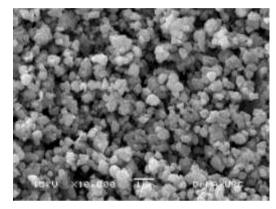
Figure 5 SEM image of Mg<sub>(0.5)</sub>Cu<sub>(0.2)</sub>Zn<sub>(0.3)</sub> Fe<sub>2</sub>O<sub>4</sub> (800°C) sample
