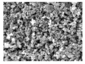
Figure 6 SEM image of g<sub>(0.5)</sub>Cu<sub>(0.3)</sub>Zn<sub>(0.2)</sub>Fe<sub>2</sub>O<sub>4</sub> (800°C) sample
