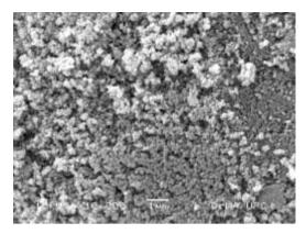
Figure 3 SEM image of  $Mg_{(0.5)}Zn_{(0.5)}Fe_2O_4$  Figure 4 SEM image of  $Mg_{(0.5)}Cu_{(0.1)}Zn_{(0.4)}$ (800°) sample
