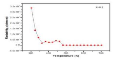
Figure 9 (b) Temperature dependent resistivity curves for  $Mg_{(0.5)}Cu_{(x)}Zn_{(0.5-x)}Fe_2O_4$  with Cu content (x=0.2)
