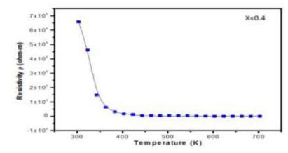
**Figure 9 (d)** Temperature dependent resistivity curves for Mg<sub>(0.5)</sub>Cu<sub>(x)</sub>Zn<sub>(0.5-x)</sub>Fe<sub>2</sub>O<sub>4</sub> with Cu content (x=0.4)
