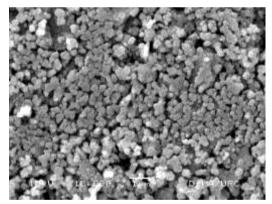
Figure 8 SEM image of Mg<sub>(0.5)</sub>Cu<sub>(0.5)</sub>Fe<sub>2</sub>O<sub>4</sub> (800°C) sample
