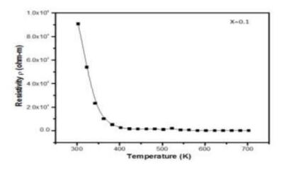
Figure 9 (a) Temperature dependent resistivity curves for  $Mg_{(0.5)}Cu_{(x)}Zn_{(0.5-x)}Fe_2O_4$  with Cu content (x=0.1)
