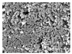
**Figure 7** SEM image of Mg<sub>(0.5)</sub>Cu<sub>(0.4)</sub>Zn<sub>(0.1)</sub> Fe<sub>2</sub>O<sub>4</sub> (800°C) sample
