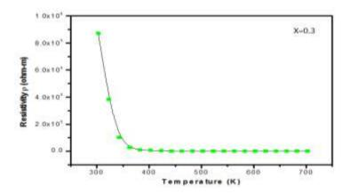
Figure 9 (c) Temperature dependent resistivity curves for  $Mg_{(0.5)}Cu_{(x)}Zn_{(0.5-x)}Fe_2O_4$  with Cu content (x=0.3)
